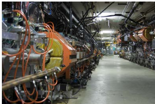
Figure 22.25 The Fermilab facility in Illinois has a large particle accelerator (the most powerful in the world until 2008) that employs magnetic fields (magnets seen here in orange) to contain and direct its beam. This and other accelerators have been in use for several decades and have allowed us to discover some of the laws underlying all matter. (credit: ammcim, Flickr)
