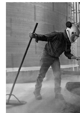
F5.24a. A worker with protective breathing gear unloads a truckload of barley. The 1000 $ helmet is battery powered with filters.
