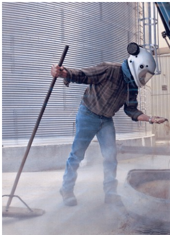
F5.24a. A worker with protective breathing gear unloads a truckload of barley. The 1000 $ helmet is battery powered with filters.
