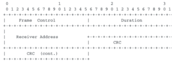
Figure 6.35: IEEE 802.11 ACK and CTS frames
